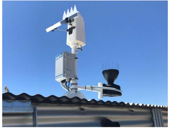
Tank Level Monitoring with added rain gauge
